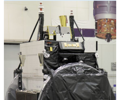
The CHIRP payload integrated on to the SES-2 spacecraft in Orbital's Satellite Manufacturing Facility
