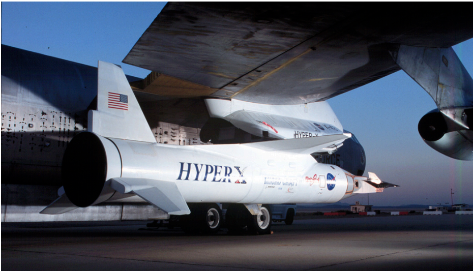
Hyper-X booster and X-43 research vehicle mated under the wing of NASA's B-52
